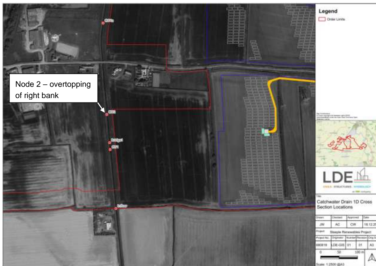
Figure 4.7: Catchwater Drain node location for single overtopping location
